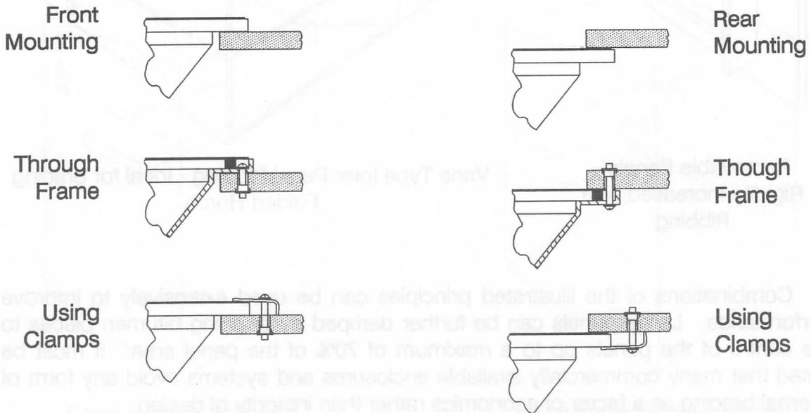
First mark out the positions of the Tee nut holes and loudspeaker cut-outs. Produce cut-out by using a power jigsaw or similar. Drill holes slightly larger than the Tee nut shank, then hammer the Tee nuts into position on the INSIDE FACE. Check that the loudspeaker fits, and the Tee nuts line up with the holes in the frame.
