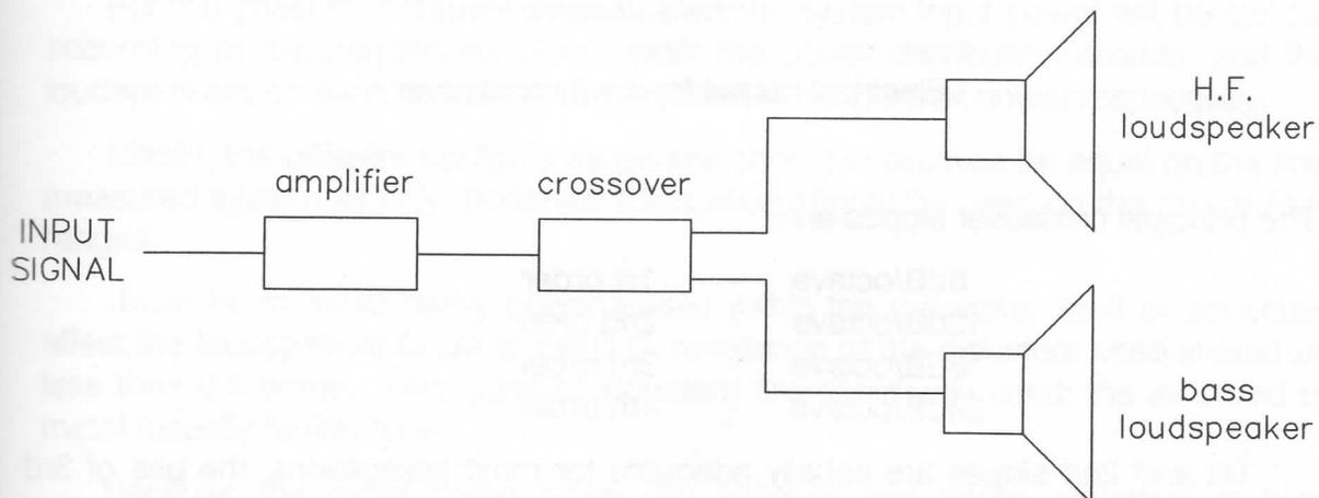
Apart from single diaphragm full range drivers, all loudspeaker enclosures or systems utilising multiples of loudspeakers covering different parts of the audio frequency spectrums need the input or line-signals dividing between various components.
