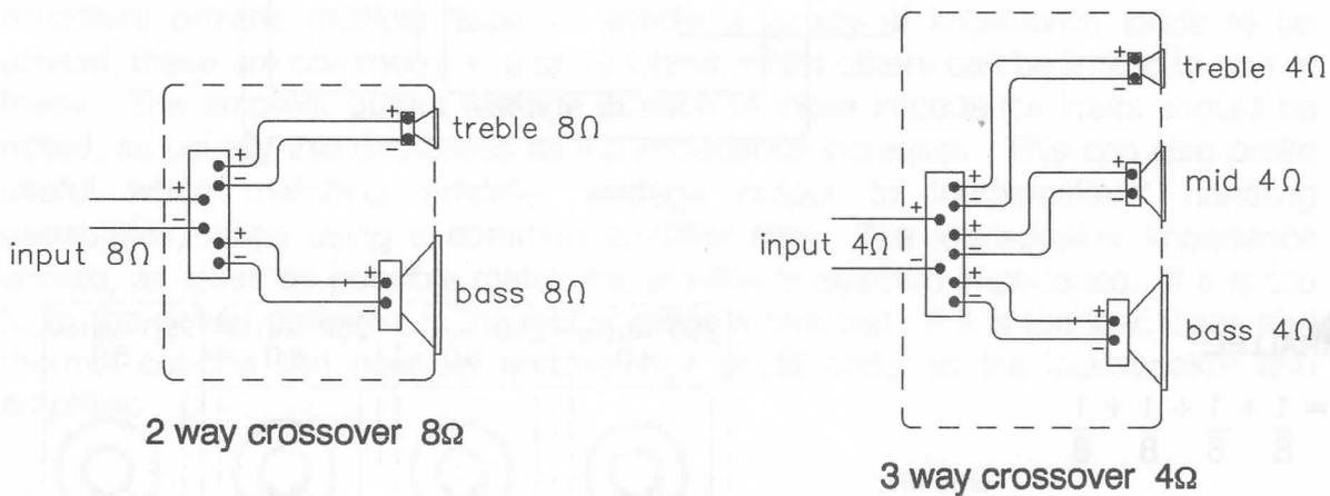
It is possible to connect more than two loudspeakers to each crossover output section, provided the stated formulae and principles are adhered to, thus maintaining the correct impedance; both loudspeakers must be of the same impedance, thereby distributing the power available equally to each.
