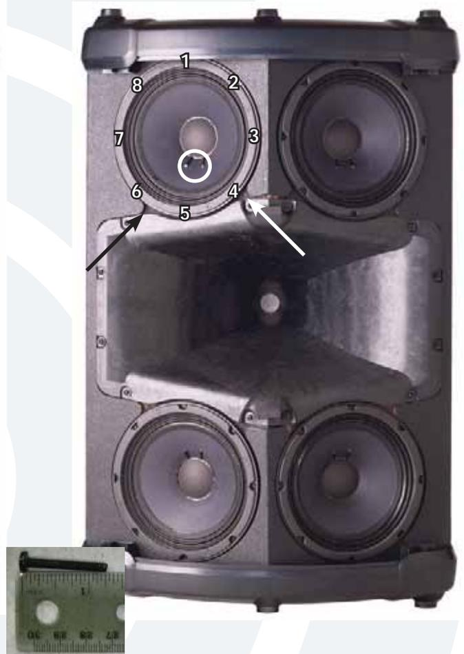
**1** Six screws need to be removed from each side of the front of the grill (twelve screws total) using the phillips head screwdriver. This grill has a tendency to want to “pop” off, so please be sure to hold it in place with one hand or arm while removing the screws with your free hand. In addition to the grill, the screws also hold the decorative trim. The trim should be removed, too. Keep the twelve screws in a safe place.
