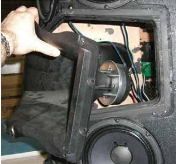
**3** Carefully begin to remove the entire horn assembly (with the high frequency driver still attached).
