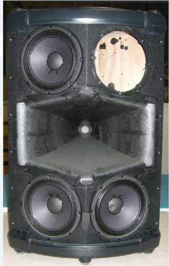
**5** The picture above shows what the S408 looks like with the grill and top right woofer removed. Place the new woofer (part #0011806) where the old one was. Follow the same steps as above, but backwards 4 to 1. Power up the S408 and the new woofer should now be pumping out glorious lows. Awesome, you just replaced an 8" woofer!
