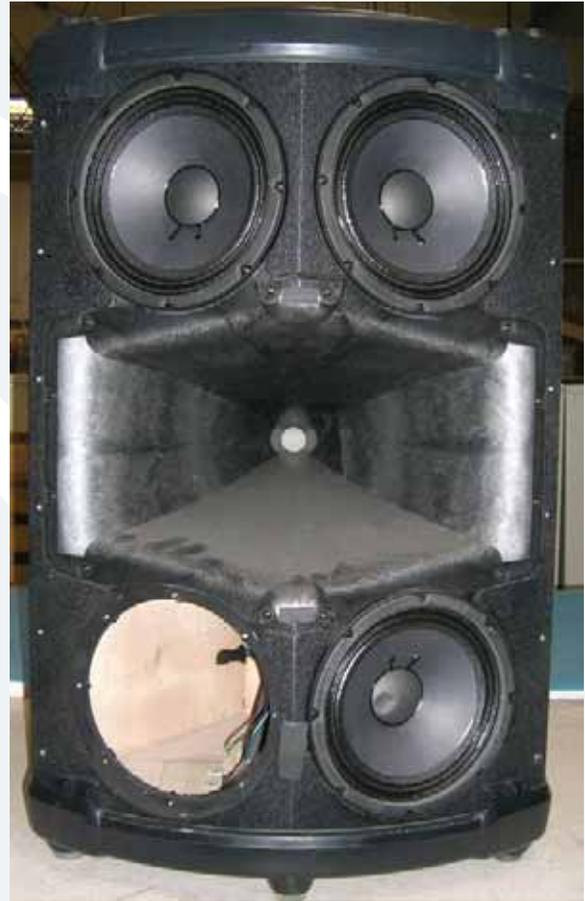
**5** The picture above shows what the S408 looks like with the grill and bottom left woofer removed. Place the new woofer (part #0011806) where the old one was. Follow the same steps as above, but backwards 4 to 1. Power up the S408 and the new woofer should now be pumping out glorious lows. Awesome, you just replaced an 8" woofer!
