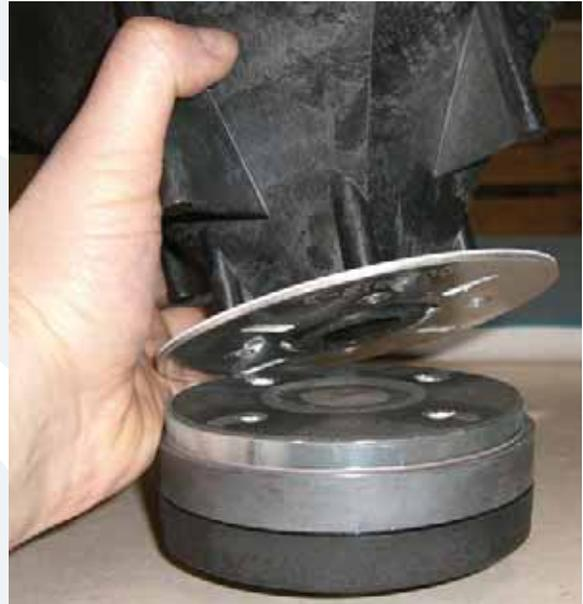
8 The horn assembly should easily lift right off of the high frequency driver. Place the new high frequency driver (part #0008093) where the old one was. Follow the same steps as above, but backwards 8 to 1. Power up the S408 and the new driver should now be pumping out those highs again. Fantastic, you just replaced a high frequency driver!
