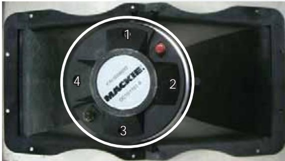
**3** The horn assembly is shown above with the high frequency driver circled. Four screws need to be removed from the driver using the 3mm allen wrench.
