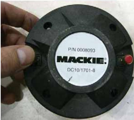
**6** This is what the plate adapter and diaphragm look like after they have been removed from the horn assembly. The diaphragm is separated from the plate adapter simply by pushing down on the terminals.
