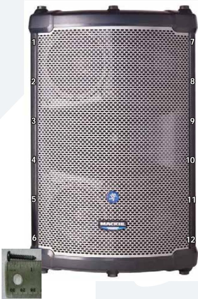
**1** Six screws need to be removed from each side of the front of the grill (twelve screws total) using the phillips head screwdriver. This grill has a tendency to want to “pop” off, so please be sure to hold it in place with one hand or arm while removing the screws with your free hand. In addition to the grill, the screws also hold the decorative trim. The trim should be removed, too. Keep the twelve screws in a safe place.
