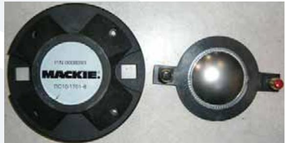
**7** This is what the plate adapter (left) and diaphragm (right) both look like. Place the new diaphragm (part # coming soon) where the old one was. Follow the same steps as above, but backwards 6 to 1. Power up the S408 and the new diaphragm should now be pumping out those highs again. Sweet, you just replaced a diaphragm!
